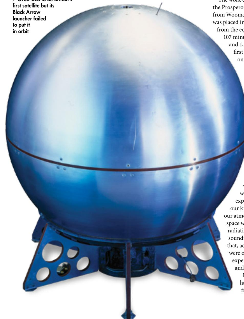
The work continued and on 28 October 1971 the Prospero satellite was successfully launched from Woomera, South Australia. The 66kg satellite was placed into an orbit with an inclination of 82° from the equator, circling the Earth once every 107 minutes, at a distance between 547km and 1,582km. Prospero had become the first and only UK satellite to be launched on a domestic rocket.
